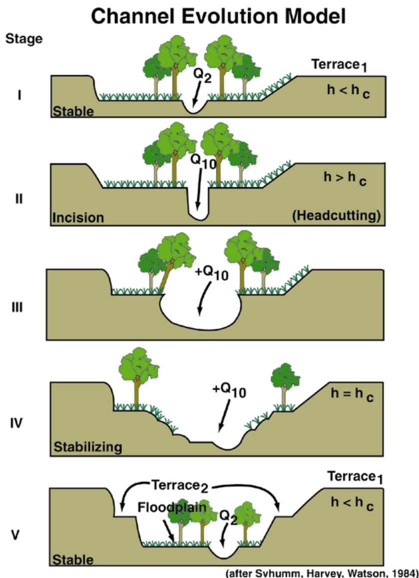
**Figure 3-9:** Stages of geomorphic evolution of an incised stream channel.
