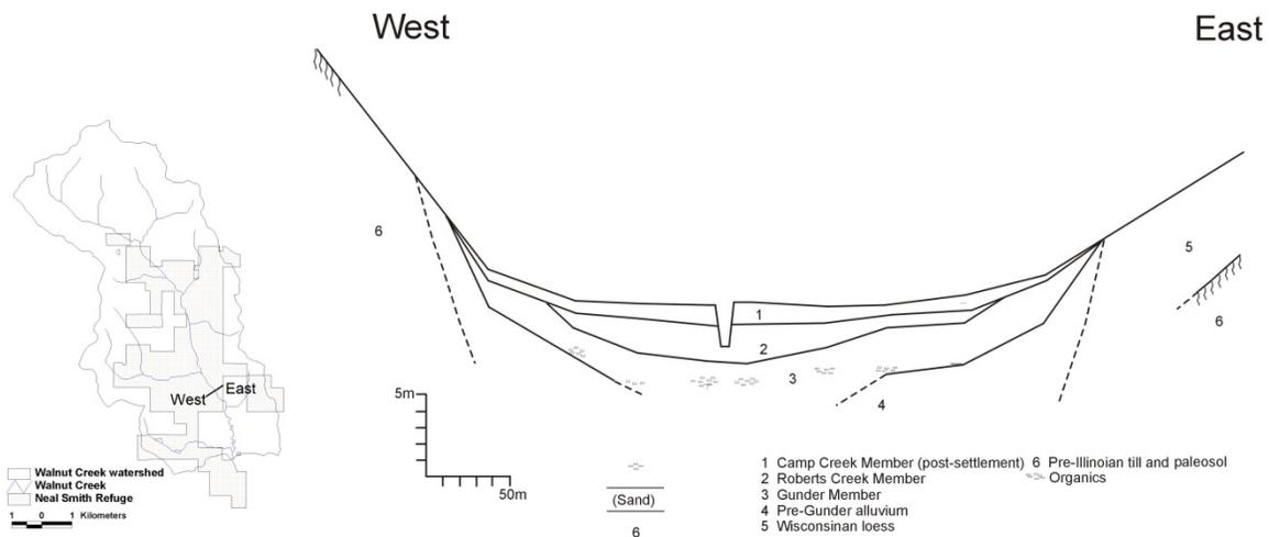
**Figure 2-3:** Cross section across the floodplain of Walnut Creek showing alluvial stratigraphy (modified from Schilling et al., 2004; Schilling et al., 2006).
