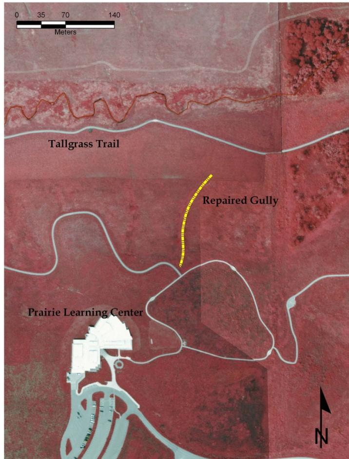
**Figure 6-1:** Experimental gully repair was accomplished with NSNWR staff and volunteers who filled a gully with waste soil and planted established plants in 2000.
