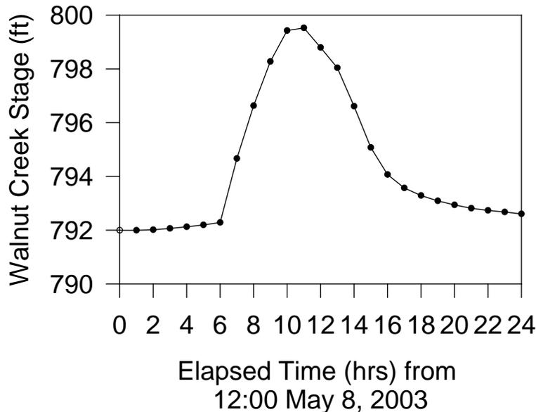
**Figure 3-10:** Hydrograph of Walnut Creek discharge that shows the flashy nature of streamflow in the incised channel. Discharge increased and decreased nearly eight feet during a 12-hour time period.
